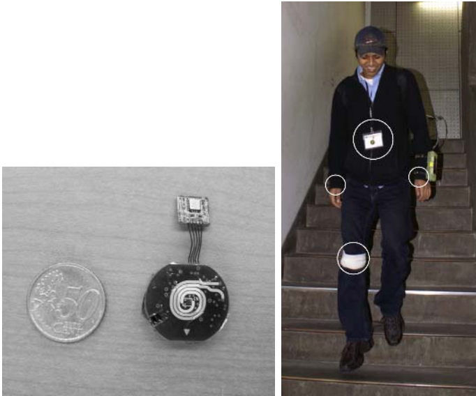
Fig. 1. The Cookie attached with three axis accelerometers (a) and placements of Cookie (b)
