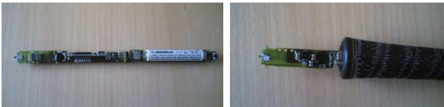
Fig. 7. The Mcard (on the left) and as partly placed into a shaft of a golf club
